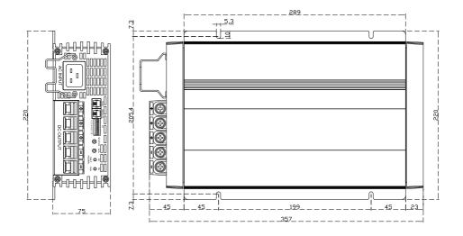
Figure 3 WSC-12120Li / WSC-2460Li / WSC-4830Li Charger Top View (mm)
