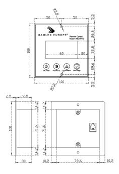
Figure 13 Remote Controller RC-601D Dimension (mm)
