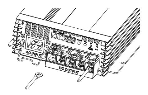
Figure 6 Cable Setup
