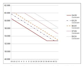
Figure 17c Temperature Compensation for 48V Model
