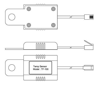
Figure 9 Temperature Sensor TF-100
