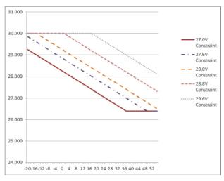
Figure 17b Temperature Compensation for 24V Model
