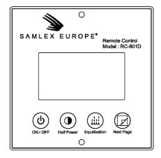
Figure 12 Remote Controller RC-601D
