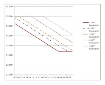
Figure 17a Temperature Compensation for 12V Model
