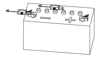
Figure 15 Temperature Sensor Setup
