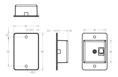
Figure 11 Remote Controller RC-600 Dimension (mm)
