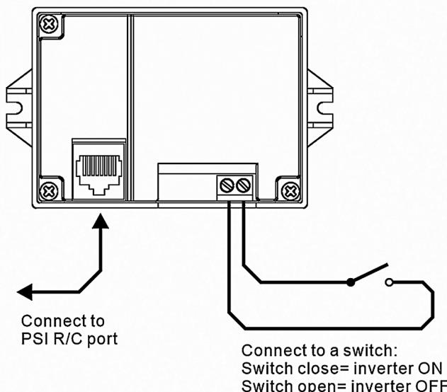
When using the remote control, ensure that the ON/OFF switch on the inverter is in OFF position
